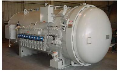
tate of the art computer control with Honeywell PLC and specifically for composite autoclaves. Features include guaranteed soak, part t/c and vacuum control, interactive screens and multilevel security.
